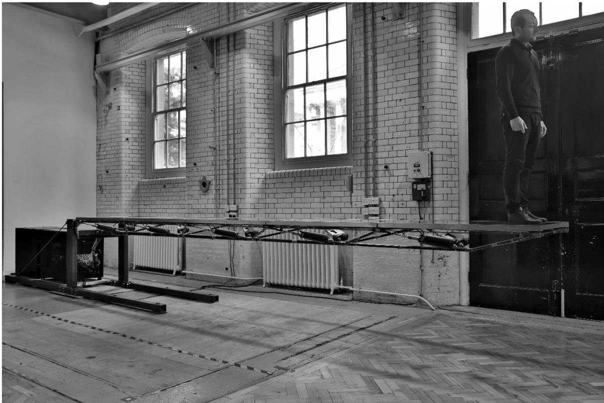
The Adaptive Truss Prototype, UCL Structures Laboratory
